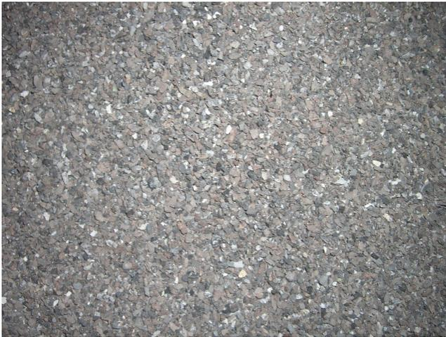
Among its many metallurgical uses, calcium carbide has been found by EAF shops to be an essential tool for the removal of unwanted iron oxide from furnace slag that is carried into the ladle during tapping. Left untreated, these oxides can interfere with the downstream steel refining operation by inhibiting desulfurization, oxidizing (“fading”) alloy additions, and attacking refractories.
